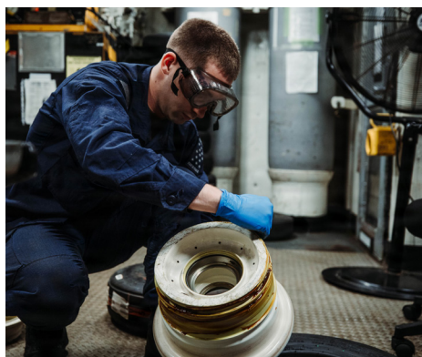
Aviation Structural Mechanic Airman Joshua Lancaster conducts maintenance on an F-18 Hornet nose mount landing gear in the tire shop aboard Nimitz-class aircraft carrier USS George Washington (CVN 73). (U.S. Navy photo by MC2 Jack Barnell)
