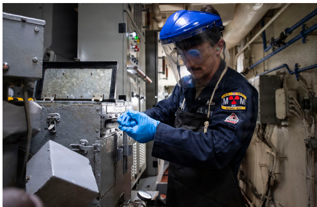
Machinist Mate 2nd Class Cory Bruno, assigned to Wasp-class amphibious assault ship USS Boxer (LHD 4), conducts daily shifting, cleaning, and inspection of lube oil strainers in the main engine room. (U.S. Navy photo by MC3 Martin Perez)
