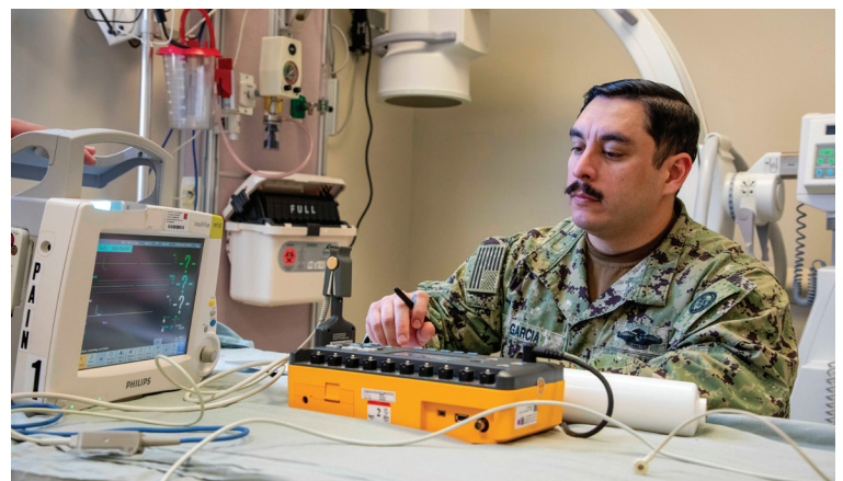
Chief Hospital Corpsman Eric Garcia, a biomedical equipment technician (BMET) with Navy and Marine Corps Force Health Protection Command (NMCFHPC) checks the diagnostics of a vital sign monitor during an annual equipment checkup for the Naval Medical Center Portsmouth, Virginia. (U.S. Navy photo by Desmond Martin)
