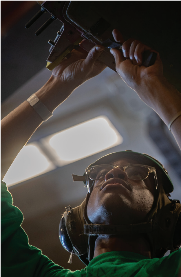
Aviation Structural Mechanic 3rd Class Ajuwon Tom, assigned to the Saberhawks of Helicopter Maritime Strike Squadron (HSM) 77, replaces sealant for blade tip caps on an MH-60R Seahawk. (U.S. Navy photo by MC2 Bruce Morgan)
