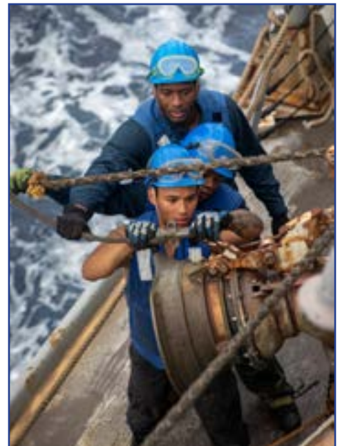
ATLANTIC OCEAN - Sailors attach span wire to a pelican hook aboard the Arleigh Burke-class guided-missile destroyer USS Bainbridge (DDG 96) during a replenishment-at-sea with the Supply-class fast combat support ship USNS Arctic (T-AOE-8).
